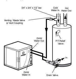
Figure 11: Hot Water Generator Installation in Preheat Tank
