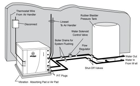
**Figure 5: Open Loop Solenoid Valve Connection Option** Typical quick operating external 24V water solenoid valve (type PPV100 or BPV100) wiring.
