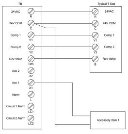
NOTES: 1) Acc Output 1 is cycled with the lead compressor 2) Acc Output 2 is cycled with the lag compressor
